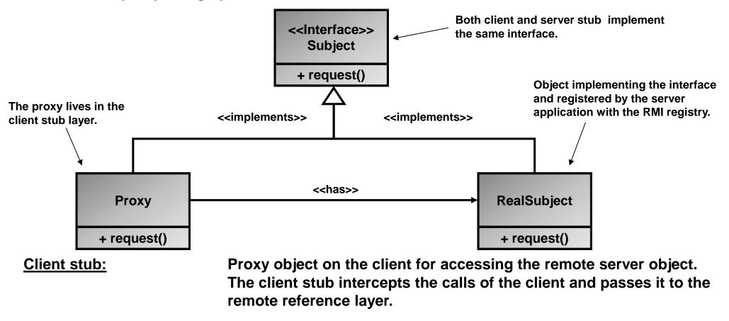
Server stub/skeleton:The server stub receives calls from the remote reference layer and<br/>passes it to the server object implementing the interface<br/>(= RealSubject in the picture above).
