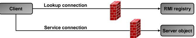
When the client fails to open a JRMP connection to the server, it automatically falls back to HTTP tunneling by encapsulating the request in an HTTP POST request.
